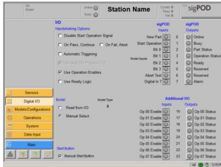
Figure 26 Digital I/O Screen – sigPOD 1608 expansion module connected
