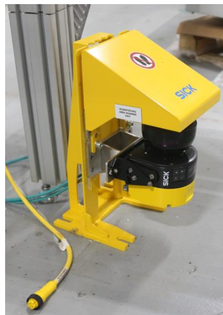
Figure 2-6. SICK Safety Laser Scanner and Heavy-duty mounting kit.
