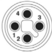
Figure 4 3520 connector: Socket M12 4-pin T-code
