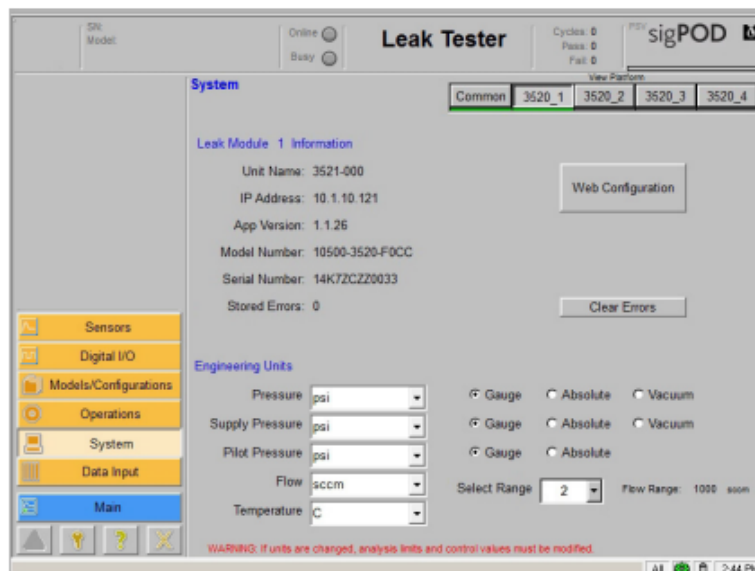
Figure 54 Example - the System screen of a 3520 leak test module
