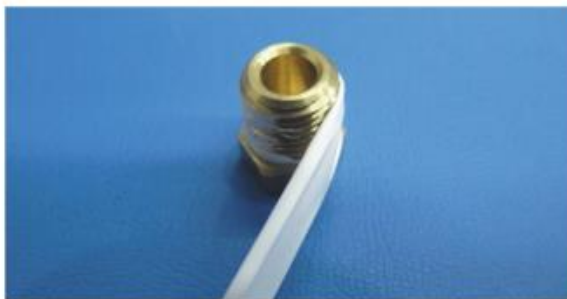
Figure 20 An example of tape correctly applied (clockwise direction) to a right-hand thread
