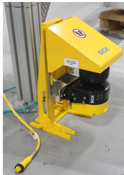
Figure 3-13. SICK Safety Laser Scanner and Heavy-duty mounting kit.
