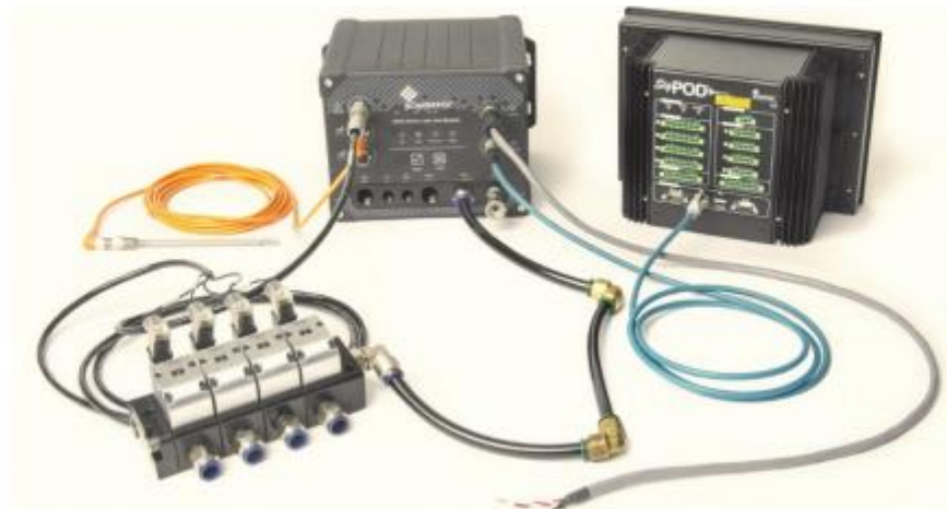
Figure 6 Example of a leak test system consisting of a 3520 C Leak Test module, a sigPOD 1200 controller, and an external valve multiplexer
