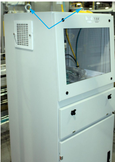
Figure 8-3. Programming terminal lifting points.
