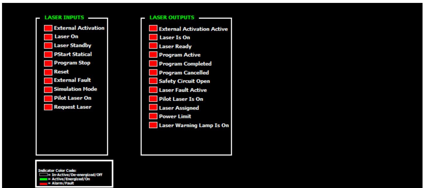
Figure 4-30. An illustration of an example Laser Handshakes screen.
