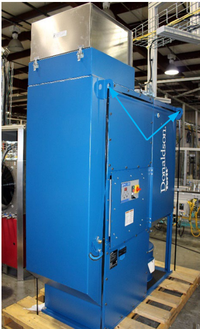
Figure 8-4. Fume extractor lifting points.
